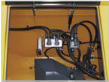
Service-friendly machine house (IP44) holding all central components in a clear and easily accessible manner. The top-hinged door provides shelter from snow and rain.
