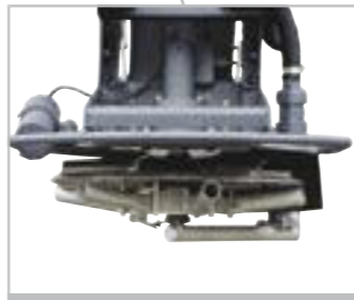
Two-sectioned spreading disc delivers dry material from the upper and liquid from the lower level via 6 special liquid pipes.
