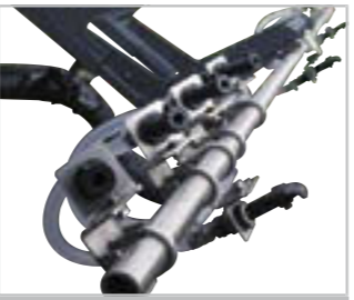
Spreading of dry material and prewetted dry material via spreading disc. Liquid is sprayed by Spratronic-nozzles making high-speed liquid spreading possible.
