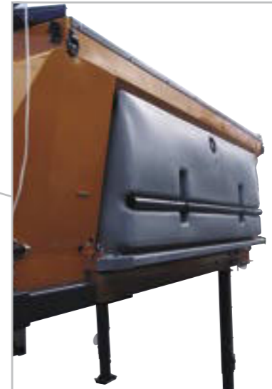
Specially designed liquid tanks for uniform filling/emptying rate.
