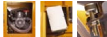
The liquid pump is a hydraulically driven diaphragm pump.
