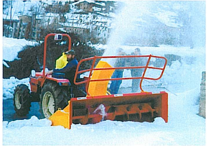
Above left: MU230 fitted to the front of a standard agricultural tractor. Above right: The MU230 fitted to the rear of a standard agricultural tractor clearing snow in northern Spain.
